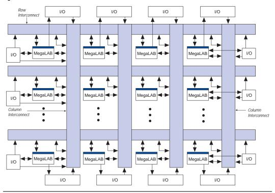
Figure 9. APEX 20K Interconnect Structure
