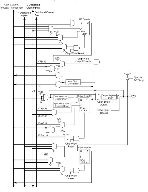
Figure 25. APEX 20K Bidirectional I/O Registers Note (1)
