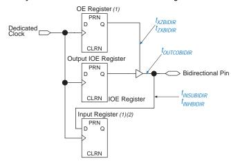
Figure 40. Synchronous Bidirectional Pin External Timing
