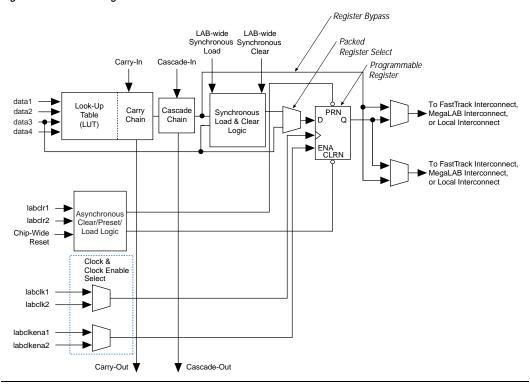
Each LE's programmable register can be configured for D, T, JK, or SR operation. The register's clock and clear control signals can be driven by global signals, general-purpose I/O pins, or any internal logic. For combinatorial functions, the register is bypassed and the output of the LUT drives the outputs of the LE.
