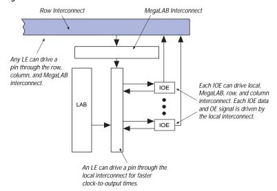
Figure 27. Row IOE Connection to the Interconnect
