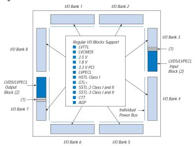
Figure 29. APEX 20KE I/O Banks
