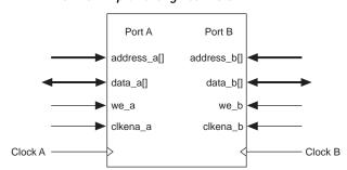
Figure 19. APEX 20K ESB Implementing Dual-Port RAM
