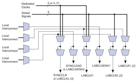
Figure 4. LAB Control Signal Generation
