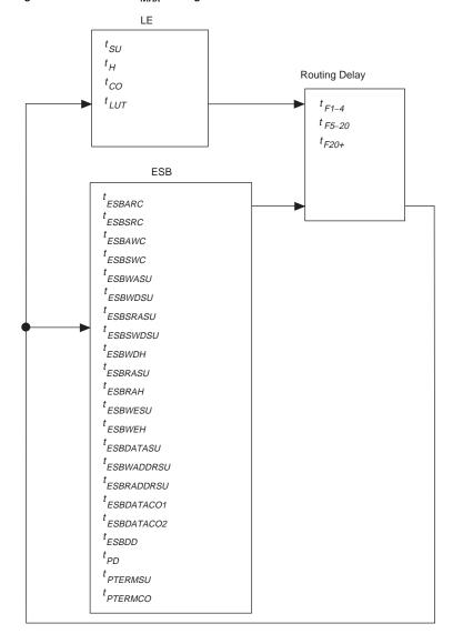
Figure 37. APEX 20KE  $f_{MAX}$  Timing Model
