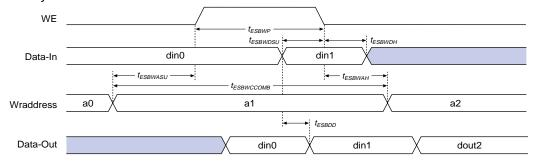
Figure 39. ESB Synchronous Timing Waveforms
